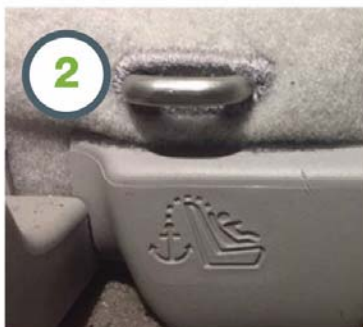
This is a tether anchor found inside the vehicle.
